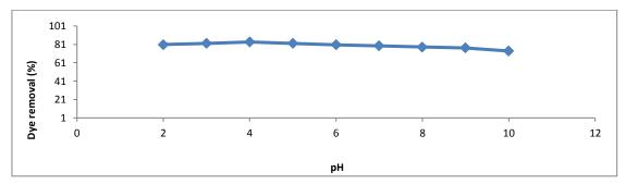
Fig. 4. Effect of pH on RB adsorption by OC (C = 20 mg/L; adsorbent dosage = 5 g/L; agitation speed=300 rpm)
