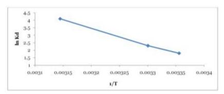
Fig. 8. Von't Hoff plot for effect of temperature on adsorption of RB onto OC.
