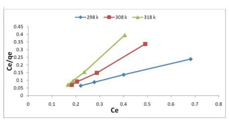
Fig. 6. Langmuir adsorption isotherm plots for adsorption of RB onto OC at different temperatures.
