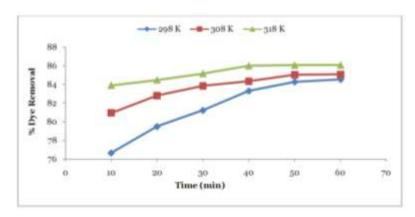
**Fig. 3.** Effect of temperature on RB adsorption by OC (C = 20 mg/L; adsorbent dosage = 5g/L; agitation speed=300 rpm).
