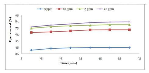
**Fig. 2.** Effect of contact time on adsorption of RB by OC at different initial dye concentration (adsorbent dosage = 5g/L; agitation speed = 300 rpm; temperature=25°C).
