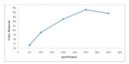
**Fig. 5.** Effect of agitation speed on adsorption of RB onto OC (C = 20mg/L; contact time = 60 min; temperature = 25°C; adsorbent dosage = 5 g/L).
