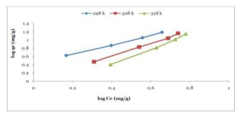
Fig. 7. Freundlich adsorption isotherm plots for adsorption of RB onto OC at different temperatures.
