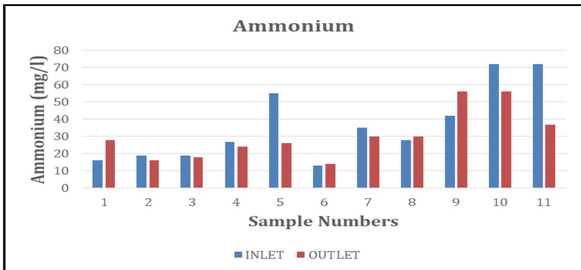
**Fig. 9.** Change in ammonium concentration of samples during domestic wastewater treatment in lab scale ABR.
