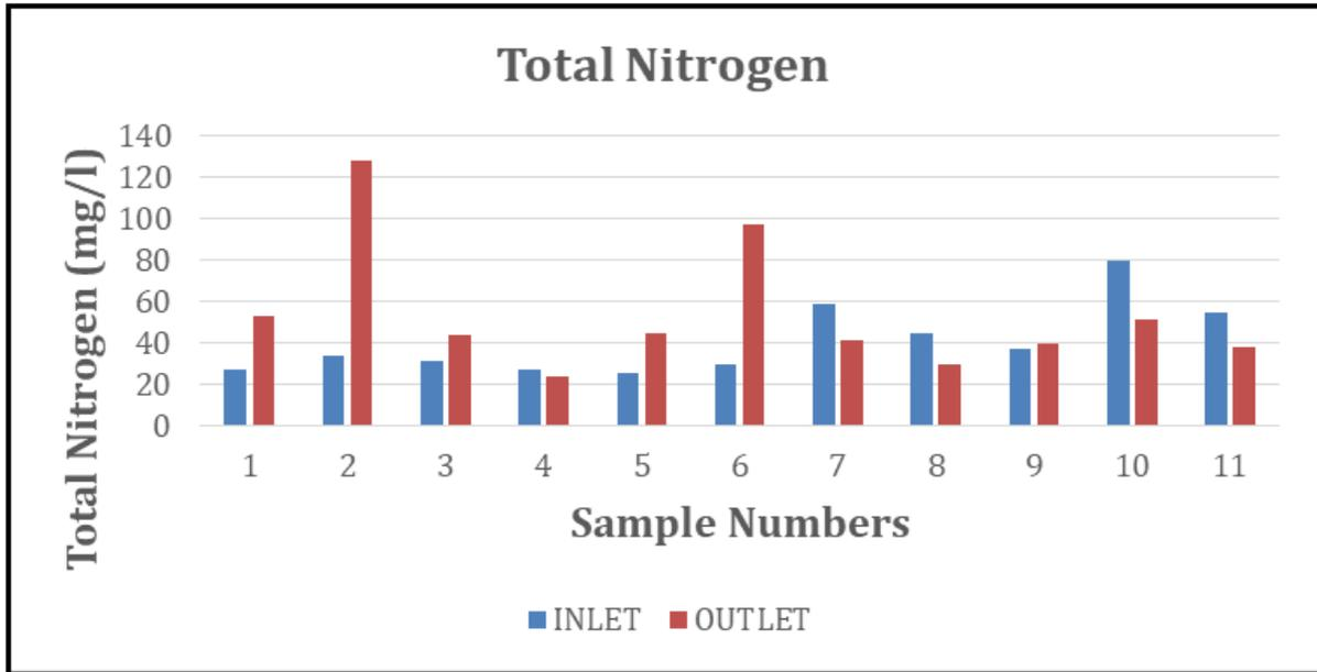
Fig. 7. Change in total nitrogen concentration of samples during domestic wastewater treatment in lab scale ABR.
