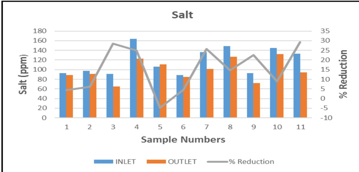
Fig. 5. Salinity of domestic wastewater before and after treatment in ABR.
