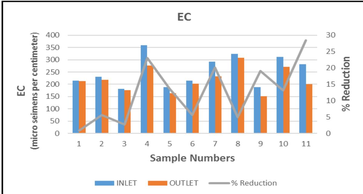
Fig. 3. EC of domestic wastewater before and after treatment in ABR.
