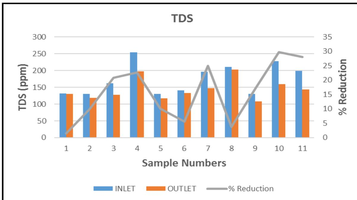
Fig. 4. TDS of domestic wastewater before and after treatment in ABR.
