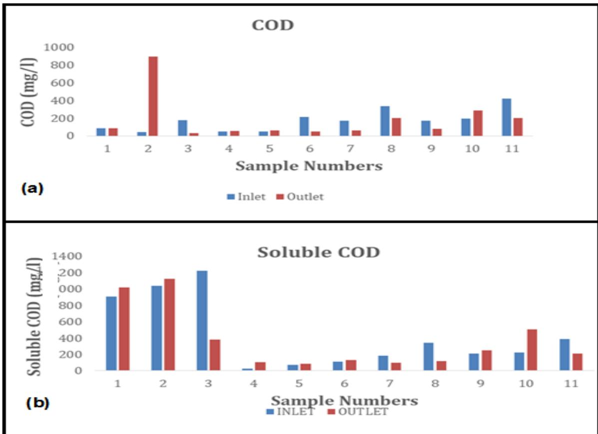
Fig. 6. Change in COD (a) and Soluble COD (b) concentration of samples during domestic wastewater treatment in lab scale ABR.
