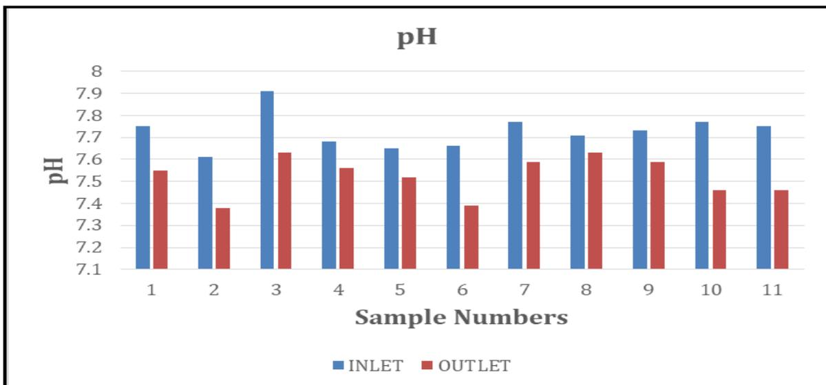
Fig. 2. Change in pH value of domestic wastewater during treatment in ABR.
