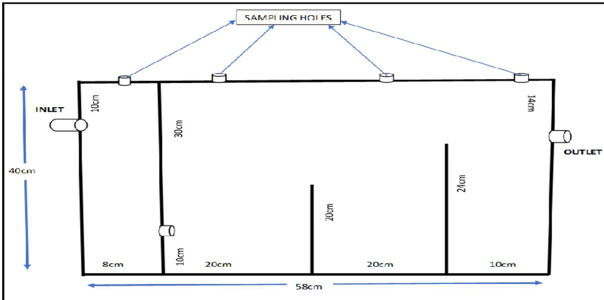
Fig. 1. Schematic Diagram of Lab scale Anaerobic Baffled Reactor (ABR).
