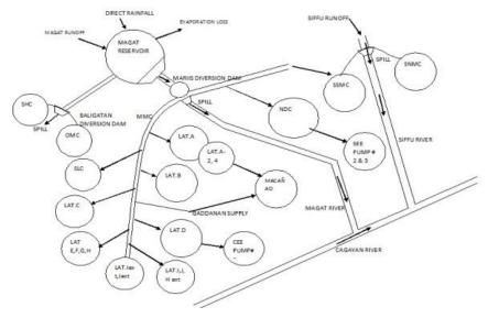
Fig. 2. Schematic layout of the NIA-MARIIS for simulation.
