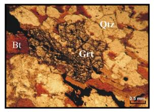
**Fig. 4.** Photomicrograph showing euhedral garnet in the melanosome part in migmatites.
