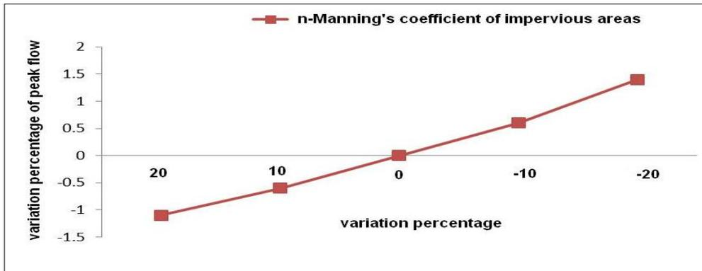
Fig. 3. variation percentage of n-Manning's coefficient of roughness in impervious areas and its effect on peak flow.
