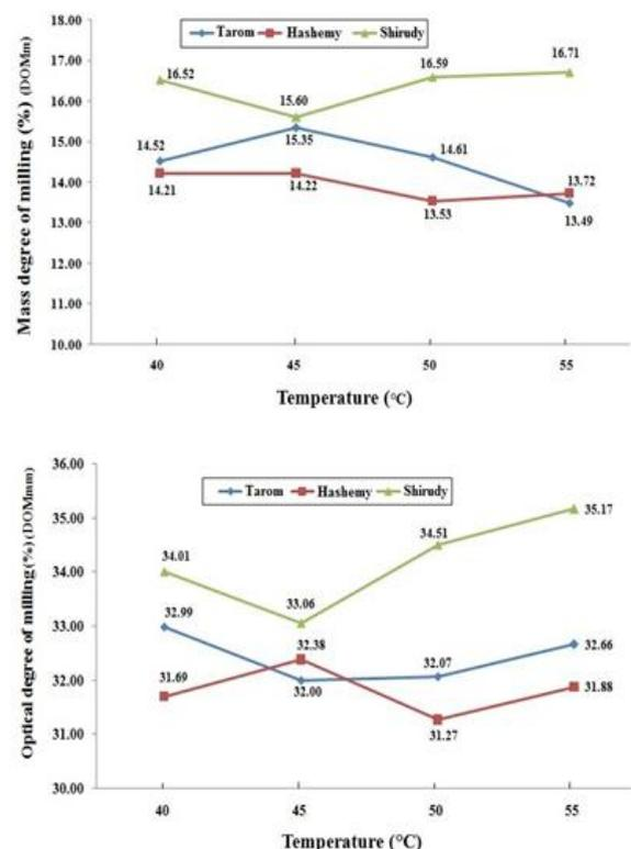
**Fig. 2.** Chart of average optical and mass degrees of milling for various varieties in different temperatures.
