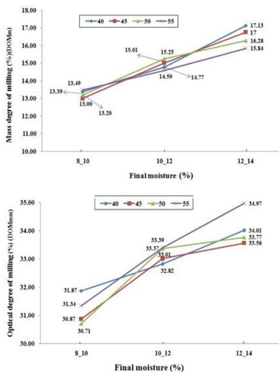
**Fig. 1.** Chart of average optical and mass degrees of milling in various temperatures for different moistures.
