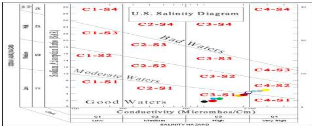
**Fig. 3.** Wilcox Diagram for Karkheh River hydrometric stations.
