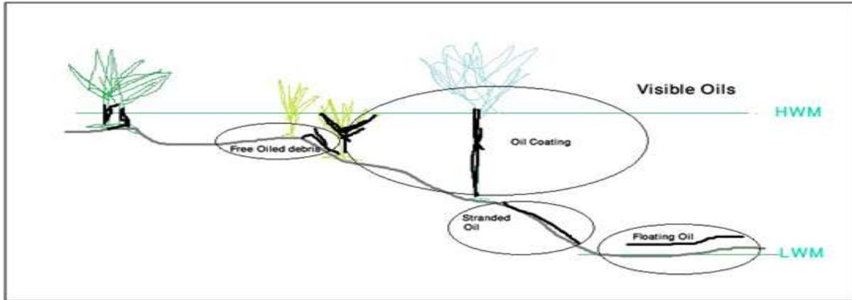
**Fig. 1.** Visible oils in the environment (HWM – high water-mark, LWM – low water-mark).
