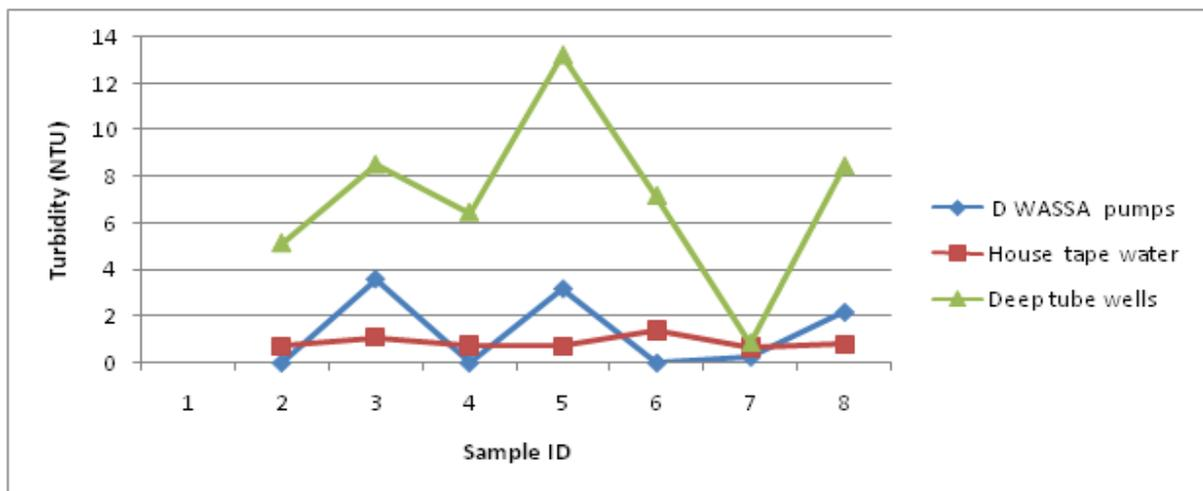
Fig. 3. Deviation of turbidity level in different water sources.
