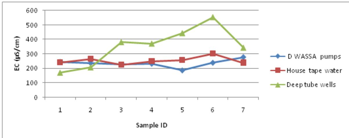
Fig. 4. Difference of Electrical conductivity in different water sources.
