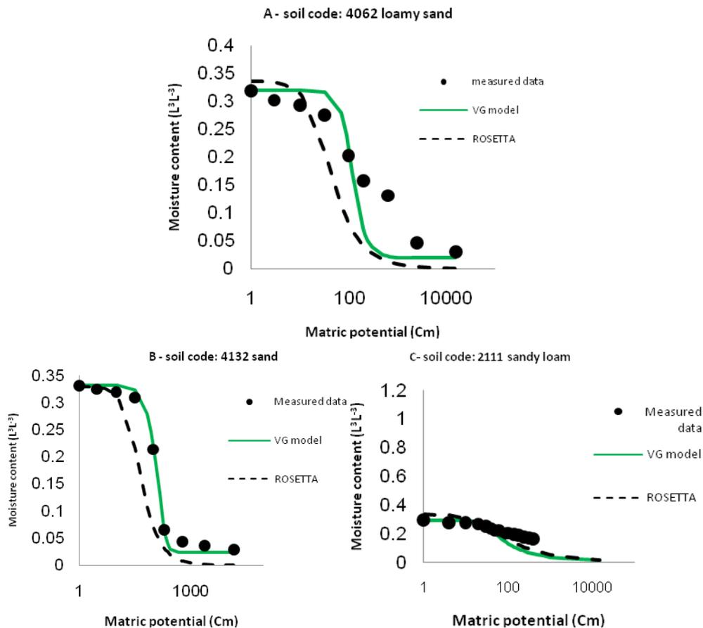
**Fig. 1.** Examples of measured and predicted water retention curve of proposed method (equation 2) and ROSETTA software for: (A) loamy sand soil, (B) sand soil and (C) sandy loam.
