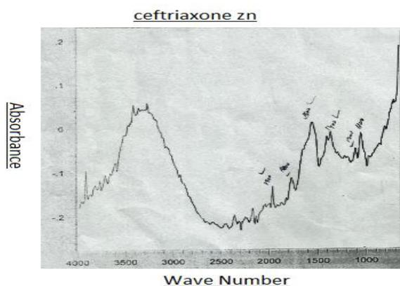
Fig. 2. IR spectra for ceftriaxone Zinc.
