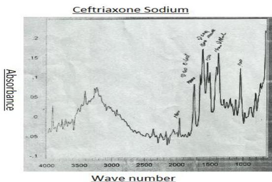
Fig. 1. IR spectra for ceftriaxone.
