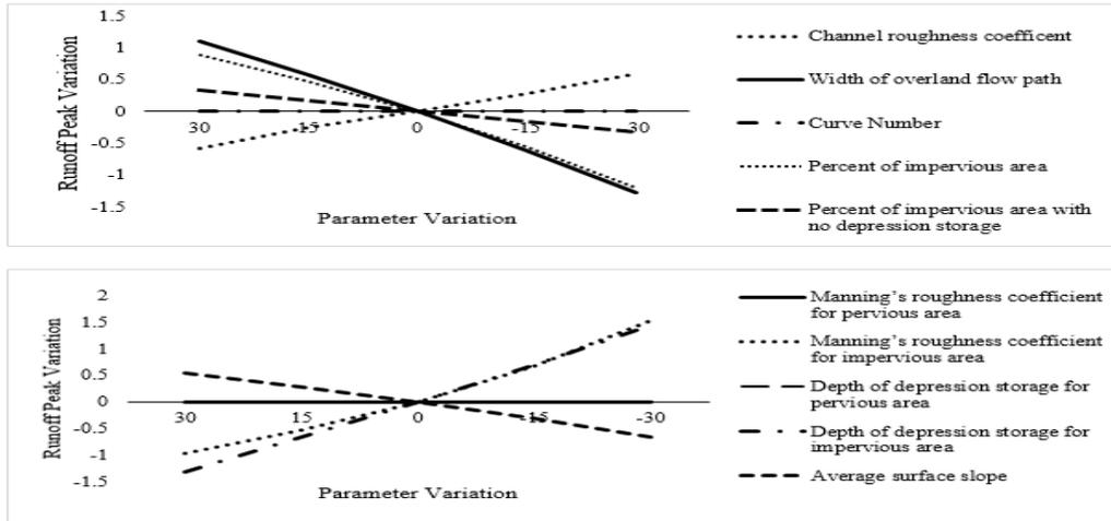
Fig. 3. The effect of SWMM model parameters change on the peak runoff.
