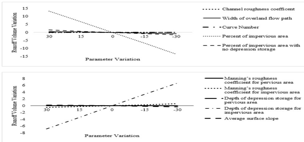
Fig. 4. The effect of SWMM model parameters change on the runoff volume.
