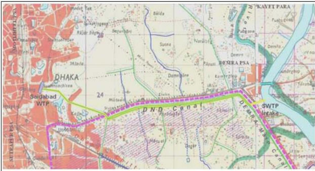
**Fig. 7.** Raw water source and its transmission network from Sitalakhya River through DND canal to SWTP.
