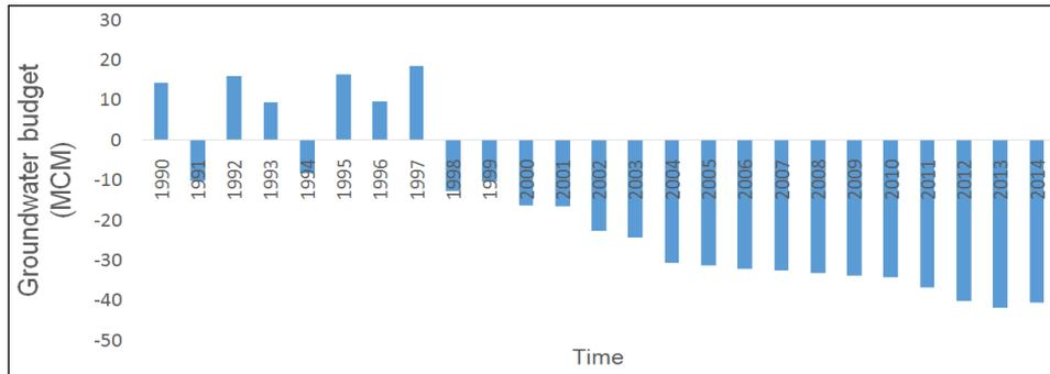
**Fig. 4.** Water budget of the study aquifer in the normal condition using MODFLOW.
