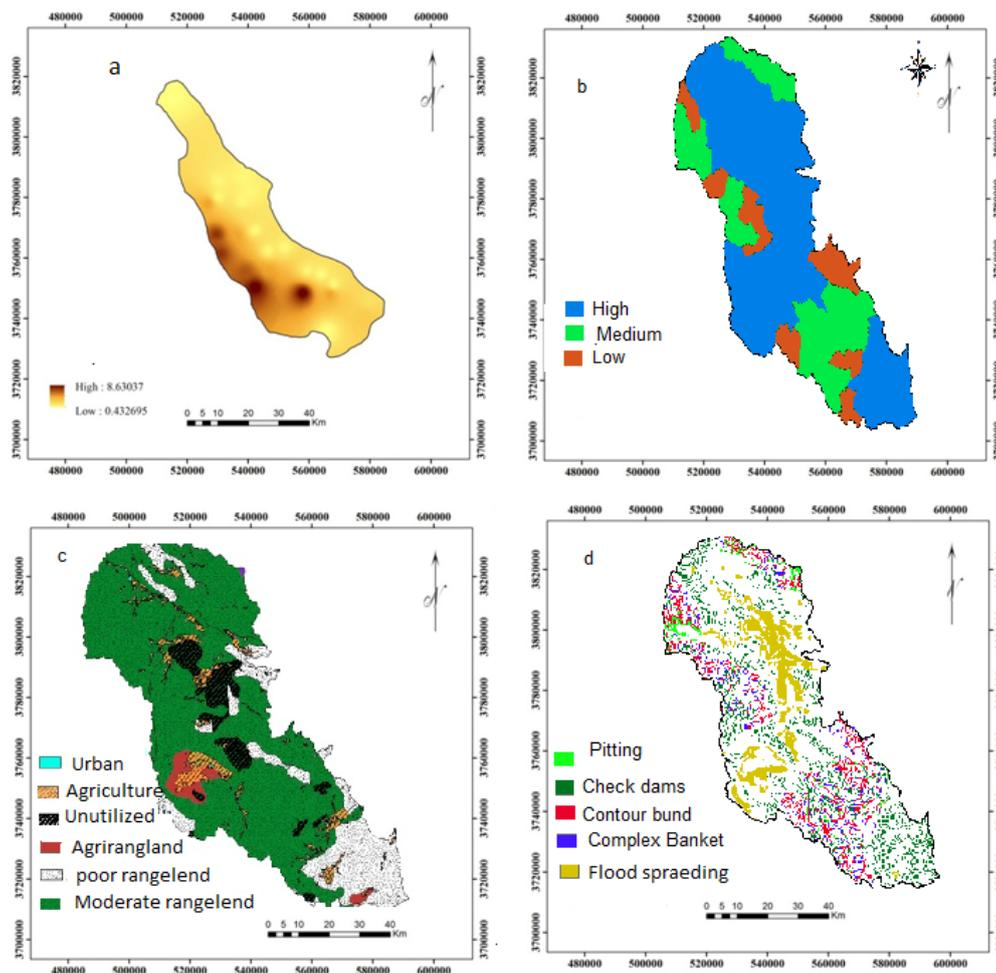
**Fig. 2.** Hydraulic conductivity of the aquifer (a); Runoff potential (b); Landuse (c) and suitable area for differences water harvesting systems (d).
