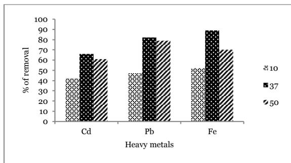
Fig. 2. Effect of temperature on biosorption.
