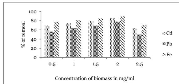
Fig. 4. Effect of biomass concentration on biosorption.
