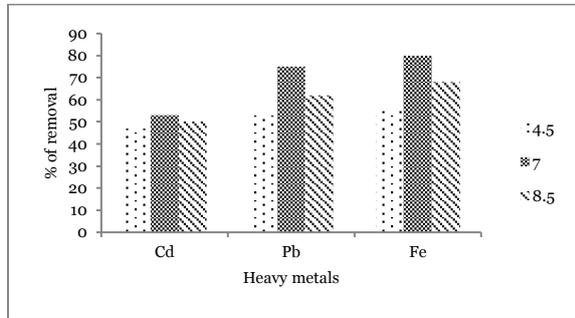
Fig. 1. Effect of pH on biosorption.
