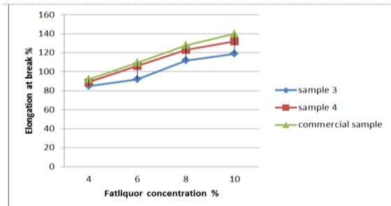
**Fig. 5.** The relation between elongation at break % and fatliquor concentration of different fatliquor samples.
