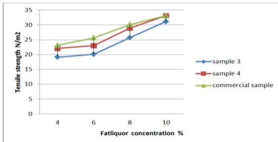
**Fig. 4.** The relation between tensile strength and fatliquor concentration of different fatliquor samples.
