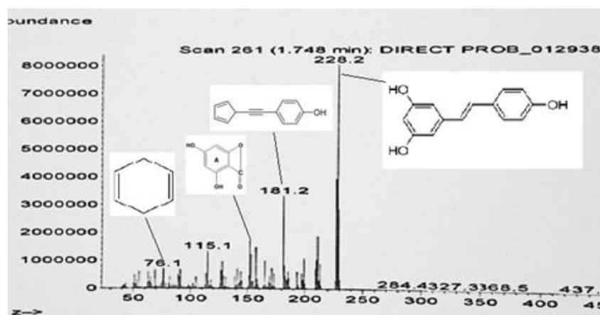
**Fig. 7.** Mass spectra of extracted pure trans-resveratrol.
