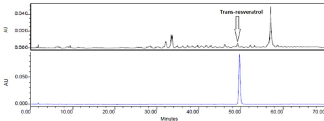
**Fig. 5.** HPLC chromatogram obtained from wild grape extracts (top) and Trans resveratrol standard (bottom) captured at 306nm.
