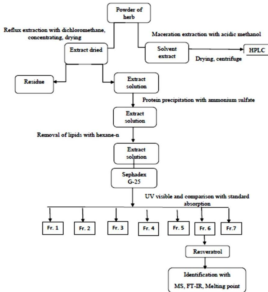
Fig. 4. Flow chart of the extraction and purification processes of resveratrol.
