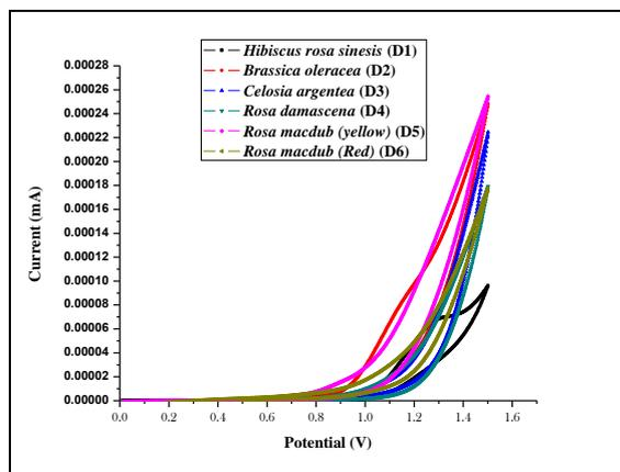
**Fig. 2.** Cyclic voltammograms of individual dye extracts of all six samples of flowers (D1-D6).
