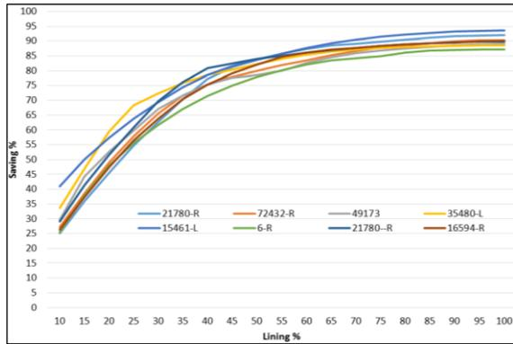
**Fig. 3.** Relationship between percent lining length & corresponding loss reduction (%).
