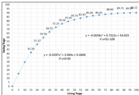
**Fig. 4.** Represents the best fit curve for relationship between percent length of lining and reduction of water-loss/salvation of lost water.
