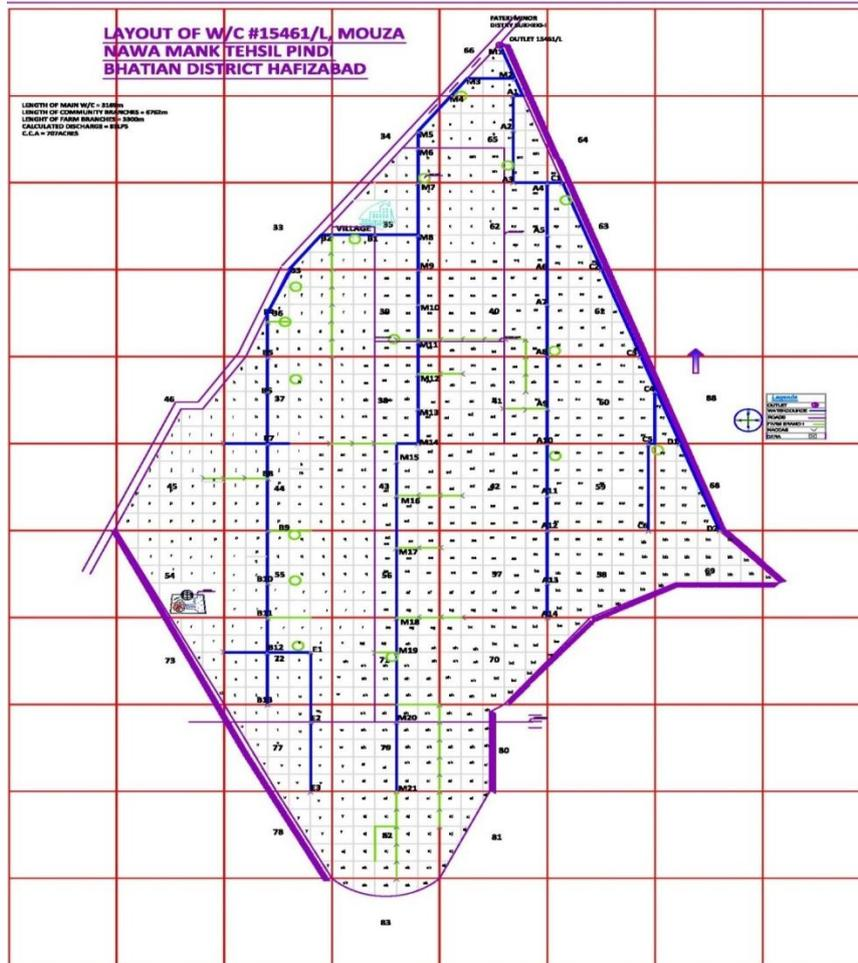
Fig. 1. Layout of a sample watercourse showing Head, Middle, Tail and flume locations.
