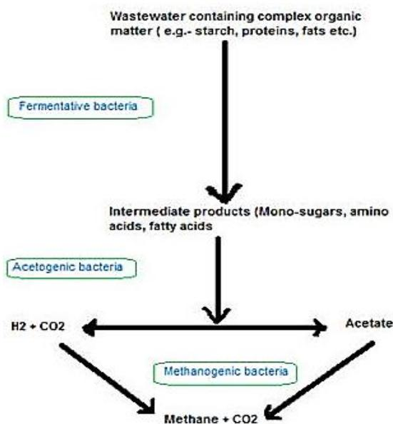
**Fig. 2.** Steps involved in anaerobic digestion process.
