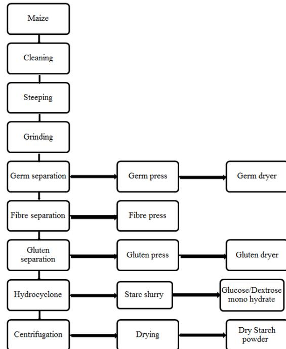
**Fig. 1.** Schematic of corn starch production by wet milling method.
