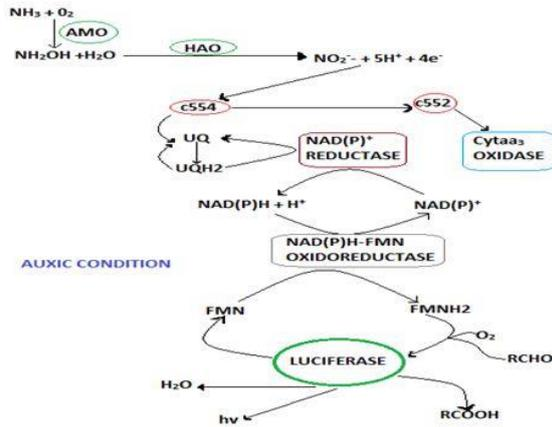
Fig. 3. Biological concept of nitrification process.
