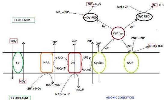
Fig. 4. Biological concept of de-nitrification process.
