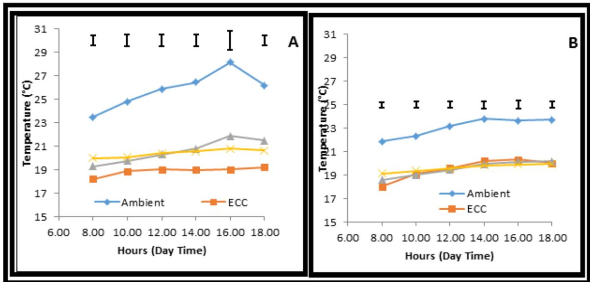
**Fig. 1.** Change in Temperature (°C) from morning to afternoon hours in Zero Energy Brick Cooler (ZEBEC), Evaporative Charcoal Cooler (ECC), Pot-in-Pot, and ambient storage for Season 1 (A) and 2 (B). Top Bars represent LSD of means ( $P \leq 0.05$ ).
