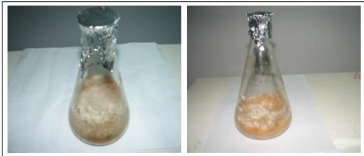
Fig. 2. Fermentation of A. niger on wheat bran as a substrate for amylase production. Fermentation was carried out at 28°C for 4 days and pH was set at 6.2.
