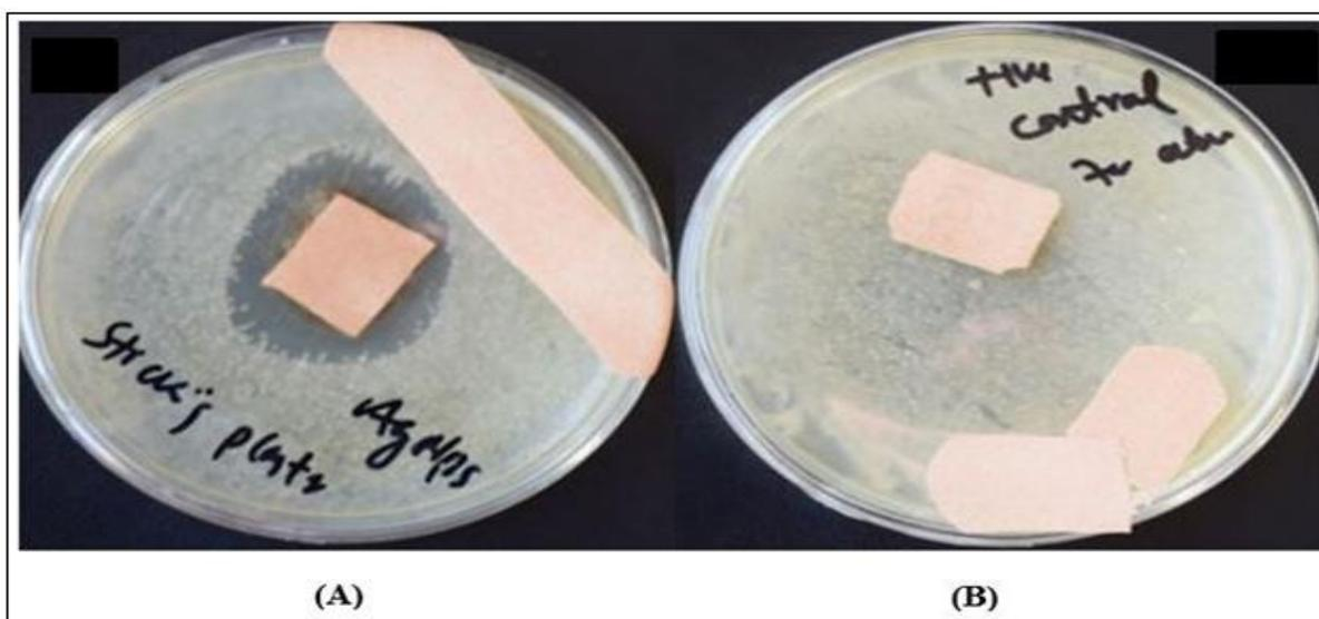
**Fig. 9.** Antimicrobial activity of AgNPs adsorbed bandage (A) AgNPs adsorbed bandage (B) Control without adsorb AgNPs.
