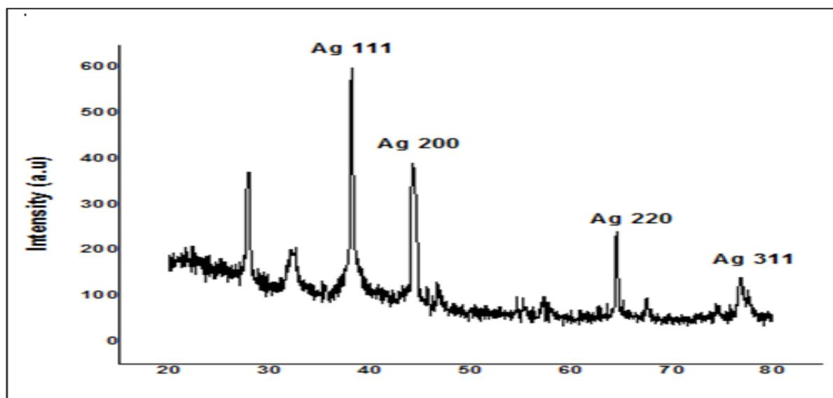
**Fig. 6.** X-ray diffraction patterns of AgNPs synthesized by using T10 bacterial strain.
