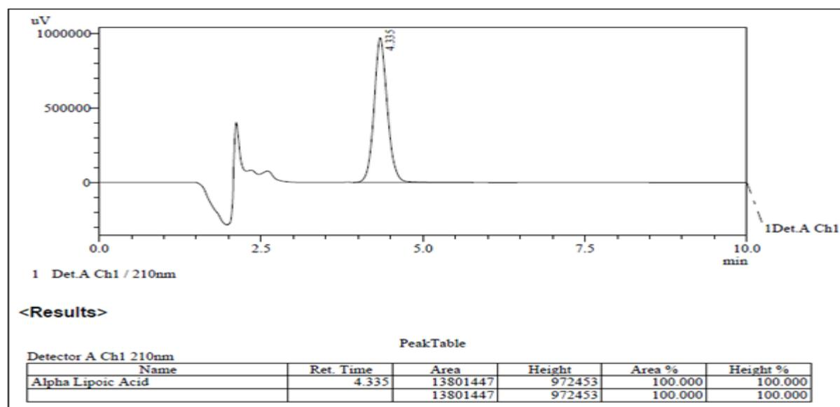
**Fig. 1.** Chromatogram of standard  $\alpha$ -lipoic acid.
