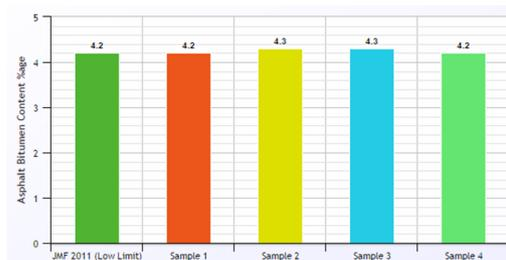
**Fig. 1.** Bitumen %age in all 4 Samples is within permissible limits of JMF 2011.
