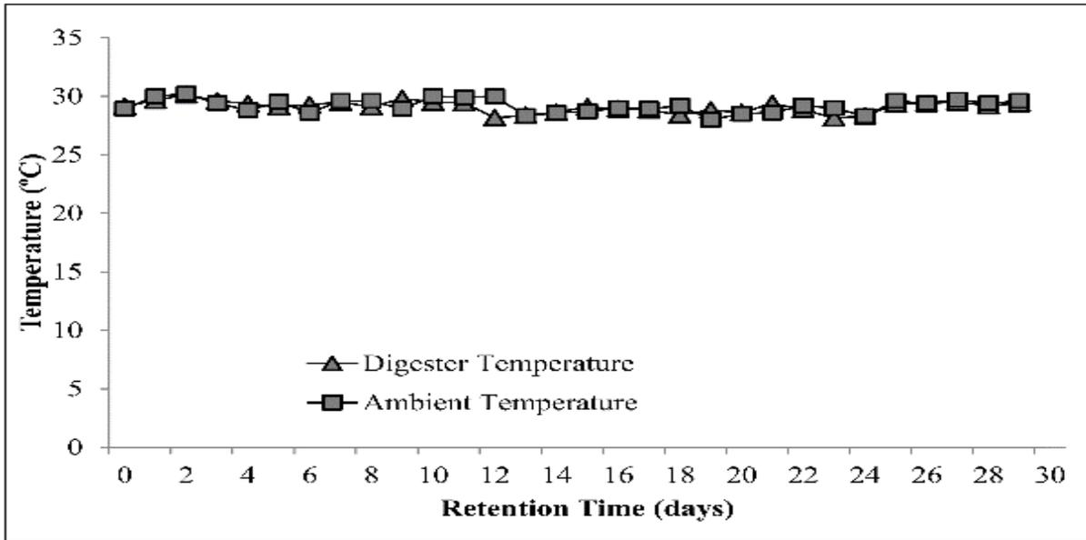
Fig. 6. The average temperature inside the digester of different particle sizes and ambient temperature.
