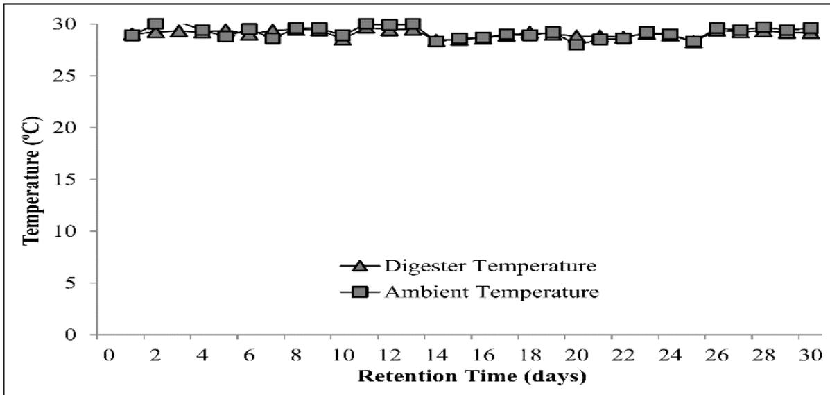
Fig. 2. The average temperature inside the digester of the vegetable wastes digester and the ambient temperature.
