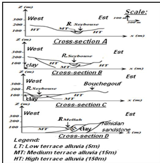
Fig. 2. Geological cross-section of the Bouchegouf plain (in Chaoui. W. 2007).
