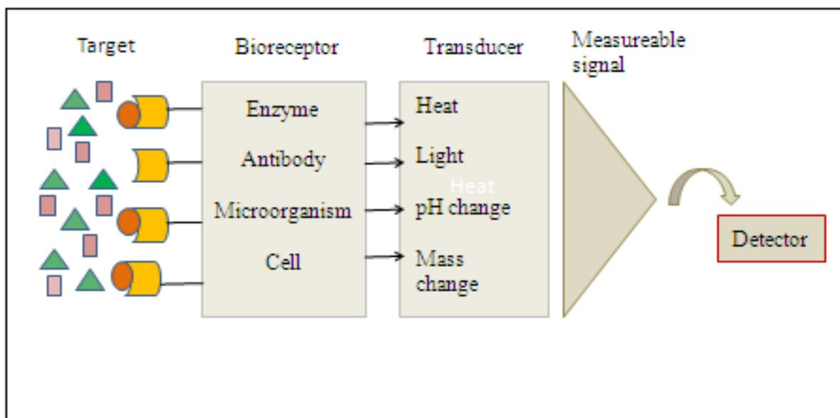
**Fig. 1.** Schematic representation of nanobiosensor.
