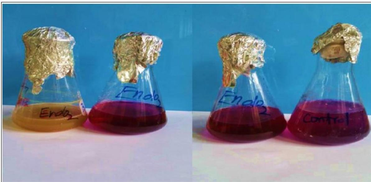
**Fig. 4.** Growth of sulphur oxidising bacteria in thiosulphate broth medium supplied with bromophenol blue use as an indicator.
