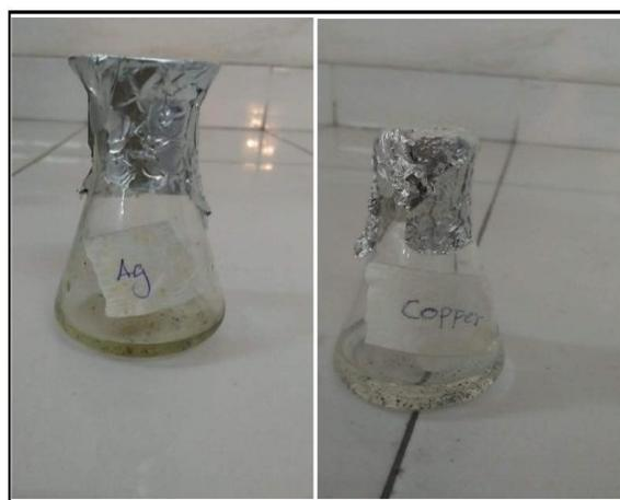
**Fig. 8.** Change in colour of DPPH solution after the addition of metal nanoparticles.
