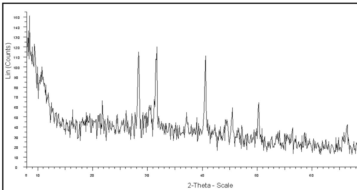
**Fig. 6.** XRD pattern of Cu- nanoparticles.
