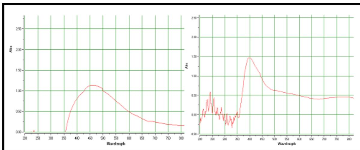
**Fig. 3.** UV Vis. Graph of Silver (left) and copper (right) nanoparticles after incubation.
