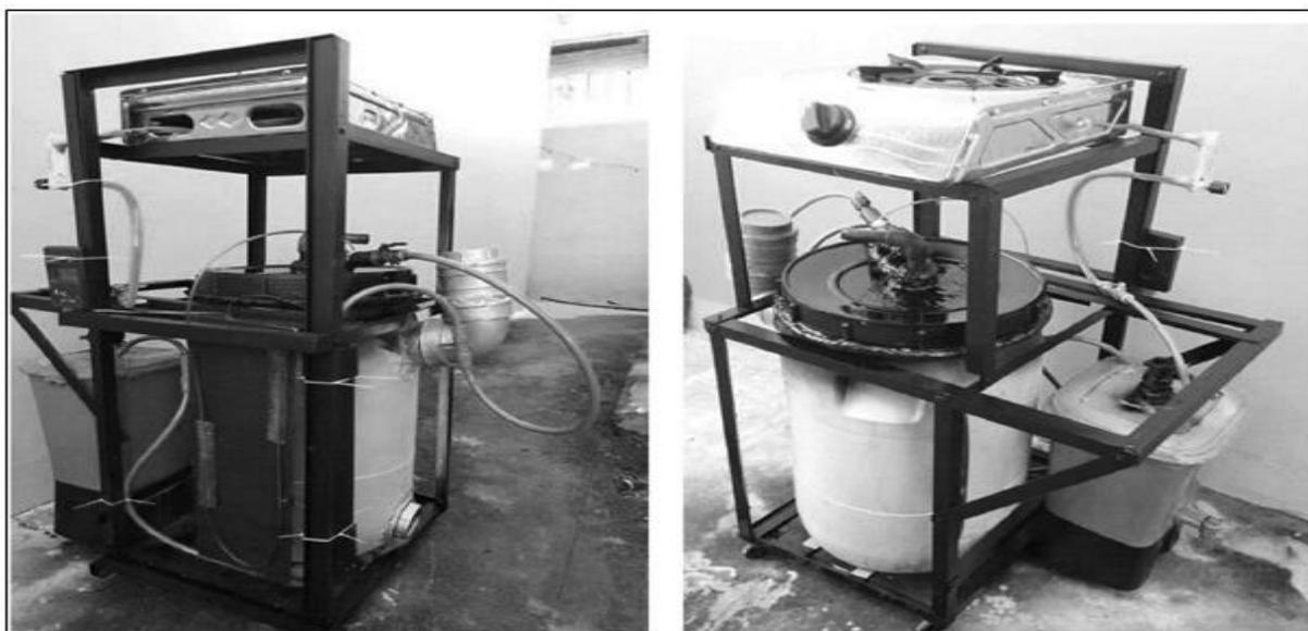
**Fig. 4.** Actual Set-up of the Portable Biogas System.
