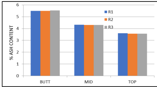
Fig. 2. Patterns for % ash content from bottom to top portion of lubeg tree species.
