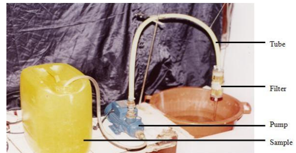
Fig. 1. Experimental disposition of the ultra-filtration mechanism with an Envirochek filter.
