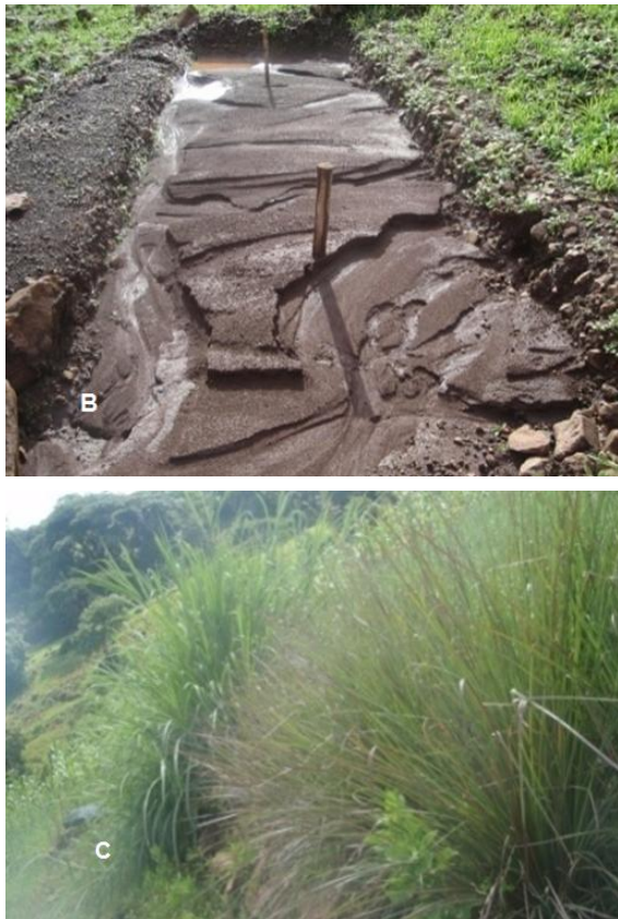
Plate 1. Field plots layout (A), sediment collection pit at the lower slope positions of the control plot (B) and grass treated bund (C).
