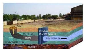
Fig. 3. Design of typical PRB (Sovani, 2005)
