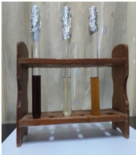
From Left to Right (A.)Synthesized gold nanoparticle in ruby red colour solution (B.) gold solution (C.) Sargassum polycystum Extract
