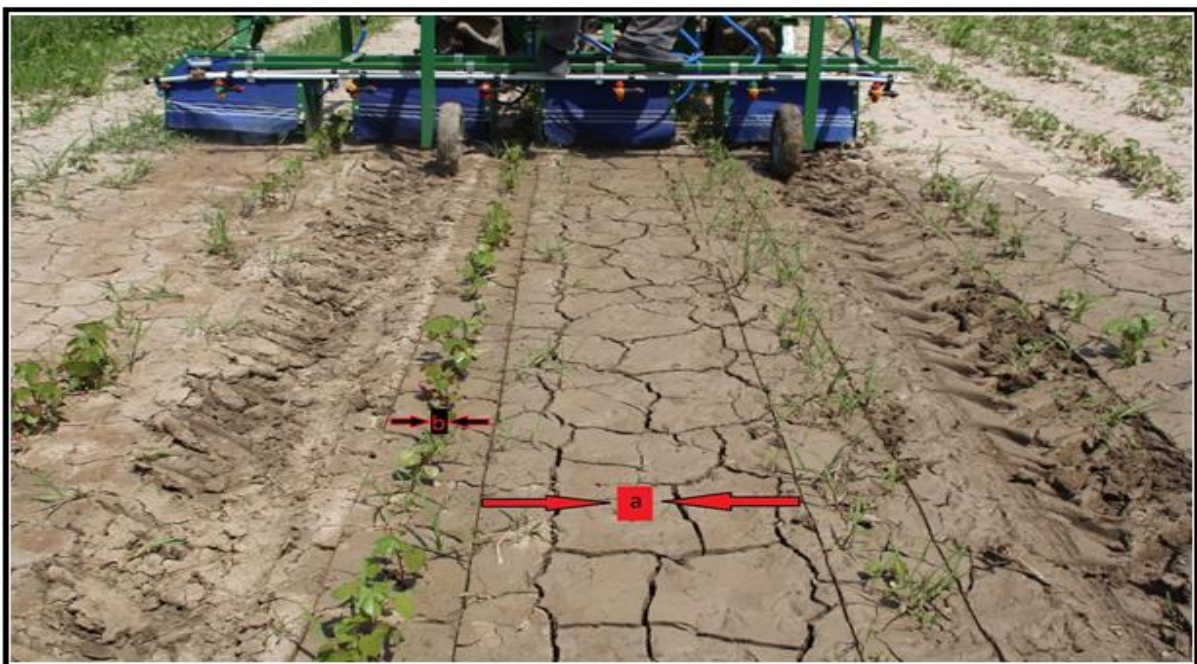
Fig. 2. Prototype of CHFS to simultaneously apply selective and total herbicides to different areas of cotton (a) to spray glyphosate inter-row weeds (b) to spray clethodim/tepraloxymid intra-row weeds.
