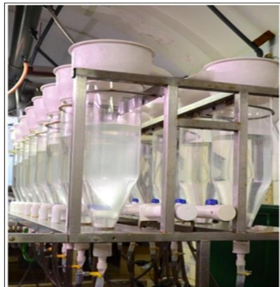
Fig. 2. Experimental set-up for mussel larvae feeding test. Sixteen 10L Zuger bottles with 5L filtered seawater and up –flow aeration system.
