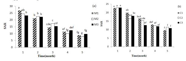
Fig. 12. SAR for three rates of (a) manure and (b)compost during 5-months incubation-leaching period.
