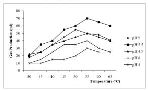
**Fig. 5.** Effect of pH and temperature on hydrogen gas production.
