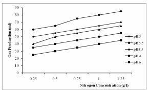
**Fig. 7.** Effect of pH and nitrogen concentration on hydrogen gas production.
