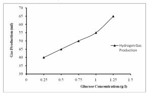
**Fig. 3.** Effect of glucose concentration on hydrogen gas production.
