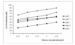
**Fig. 6.** Effect of pH and glucose concentration on hydrogen gas production.
