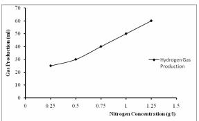
**Fig. 4.** Effect of nitrogen concentration on hydrogen gas production.
