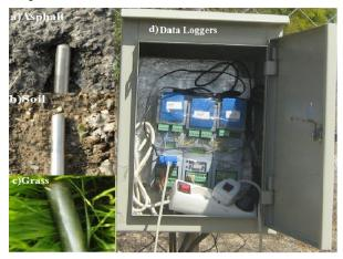
**Fig. 3.** Land covers (a) Asphalt b) soil c) Grass) and OPUS 200/ 300 Data Loggers (d).
