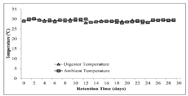
Fig. 6. The average temperature inside the digester of different particle sizes and ambient temperature.
