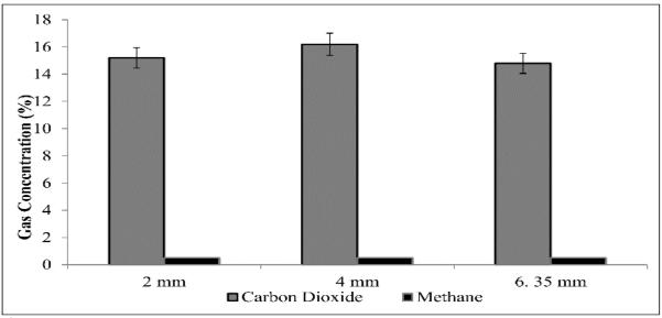
Fig. 9. Average Carbon Dioxide and methane at varying particle sizes.
