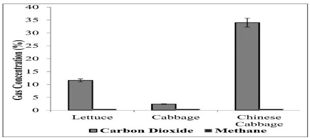
Fig. 5. Gas Concentration of each of the selected vegetable wastes.
