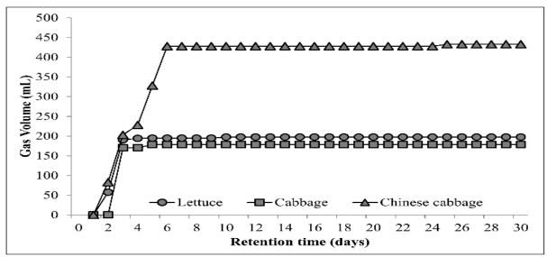
Fig. 4. Volume displacement of each of the selected vegetable wastes.
