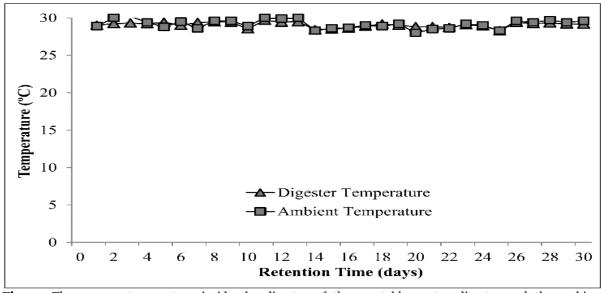
Fig. 2. The average temperature inside the digester of the vegetable wastes digester and the ambient temperature.
