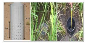
**Fig. 1.** Installed Pani pipe tube in the Experimental Are.
