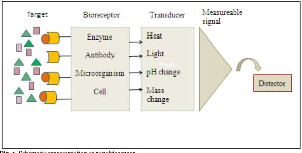
Fig. 1. Schematic representation of nanobiosensor.
