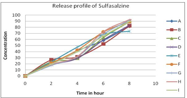
Fig. 6. Sulfasalazine release profile in simulated fluid.
