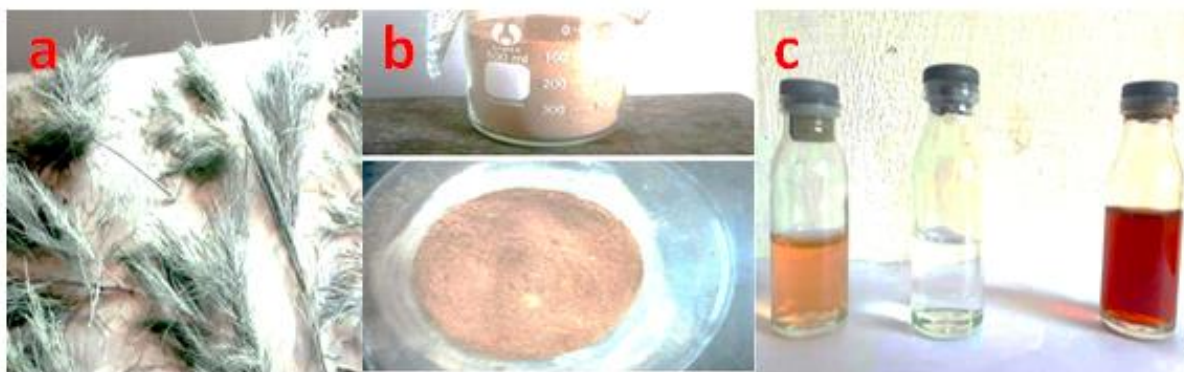
Fig. 1. (a). Drying of Tamarix Aphyllai (b): Powdered form for extraction (c): Steps involved in the synthesis of Ag-NPS.
