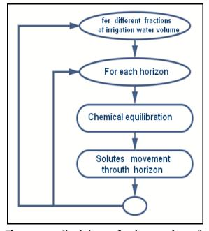
**Fig. 5.** Simulation flowchart of soils salinization/sodification process, as a result of irrigation by SMSS2 model (in Lahlou.1998) modified.
