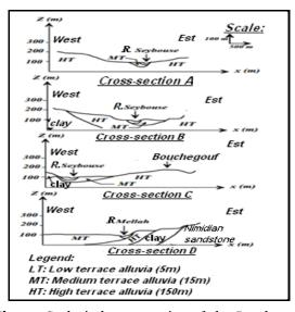
**Fig. 2.** Geological cross-section of the Bouchegouf plain (in Chaoui. W. 2007).
