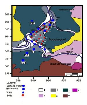
**Fig. 3.** Water and soil points Location and geological scheme of the Bouchegouf aquifers (after M. J. Flandrin 1930 modified). 1: Low terrace alluvia (5m); 2: Medium terrace alluvia (15m); 3: High terrace alluvia (150m); 4: (red Sandstone clays and conglomerates) clays greybeard and conglomerates red; 5: Numidian Sandstone; 6: Numidian clay; 7: Trias.
