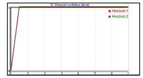
**Fig. 7.** Irrigation simulation of soil not salinized by Seybouse river water: evolution of electrical conductivity after a contribution of 7 pore volumes.
