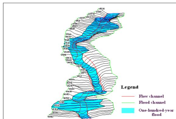
**Fig. 9.** Numerical simulation for One-hundred-year flood.
