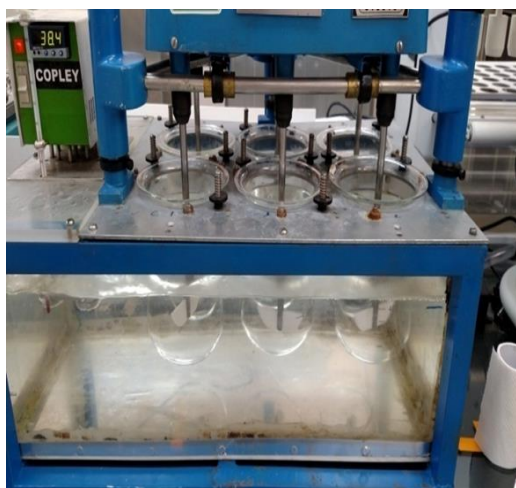
Fig. 2. Dissolution Apparatus set with the condition of normal body temperature.
