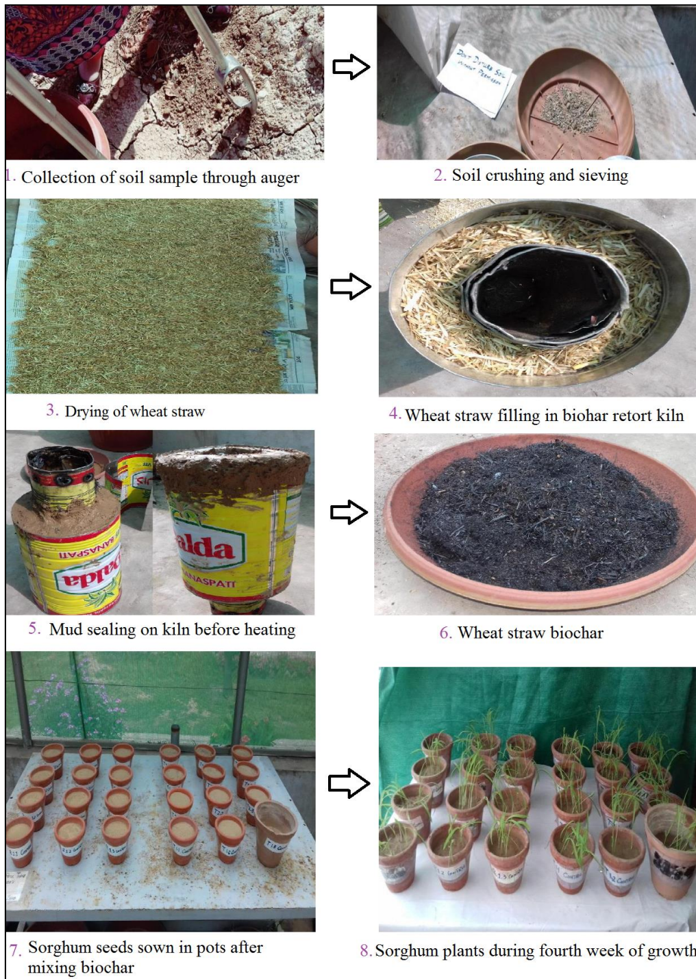
Fig. 3. Layout for biochar formation and its application in arid (Thar) and semi-arid (Rawalpindi), Pakistan soils for enhancing plant growth (Iftikhar et al. , 2018).
